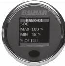
Viewing HISTORY steps the user through the minimum and maximum values recorded of the real-time data parameters. An additional set of values is shown here for POWER, expressed in watts.
