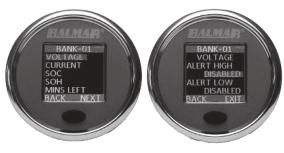
First, select the type of alert you wish to configure, then if you wish to configure for a high or low value. Once selected, you can change the value one digit at a time, using the same method used to configure the battery capacity.
