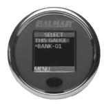
Each SmartShunt on a SmartLink Network has it's own menu. If you only have one SmartShunt, it is automatically selected for you. Otherwise, select the SmartShunt that you wish to configure (Using the long-press method) and then select MENU, and then CONFIG. A complete description of the configuration options can be found in the CONFIG section later in this manual.
