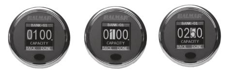
Once you select a chemistry, you must specify the capacity of the battery bank. This is the total design capacity of the entire bank, regardless of the battery's condition, or previously measured capacity. Typically the capacity is expressed as the 20-hour discharge rate. This may be written as something like "105Ah/20h" on the battery or battery documentation. If you cannot find an Ah specification for your battery, but it does show a reserve capacity (RC)
