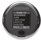
The currently selected battery type is noted with an asterisk (\*) in front of the name. The default is AGM-STD (see the chemistry table). If this is your chemistry and the installation is new, you may either re-select the chemistry, ensuring that the SG200 is starting fresh, or exit back to MENU and move to the next step.
